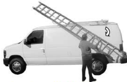
Rotate the rear of the ladder to the ground, resting front of ladder on Outer Tube
