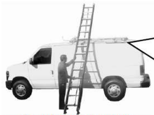
After removing ladder, return Rod Handle to the Unlocked Position in the locking mechanism.
